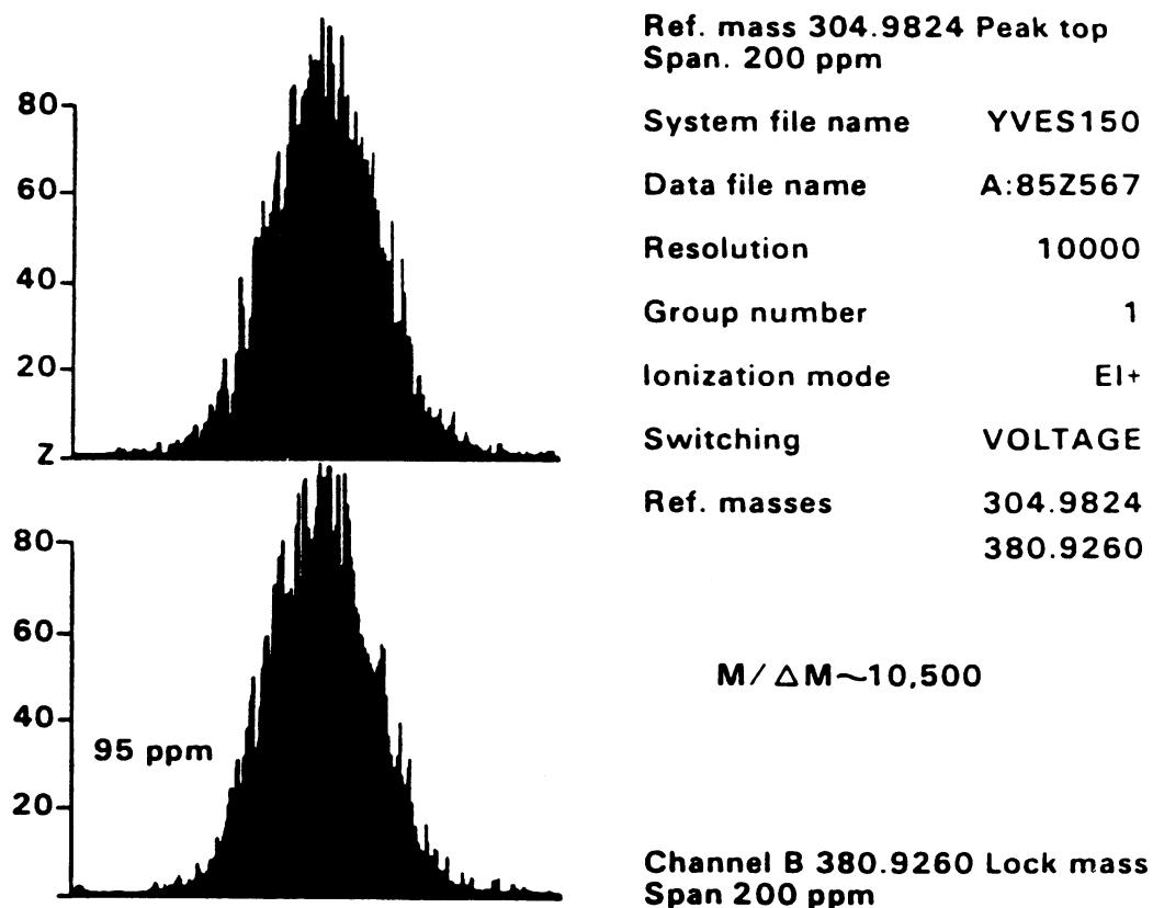
The resolution of the high-mass signal is 95 ppm at 5 percent of the peak height; this corresponds to a resolving power  $M/\Delta M$  of 10,500 (10 percent valley definition).
