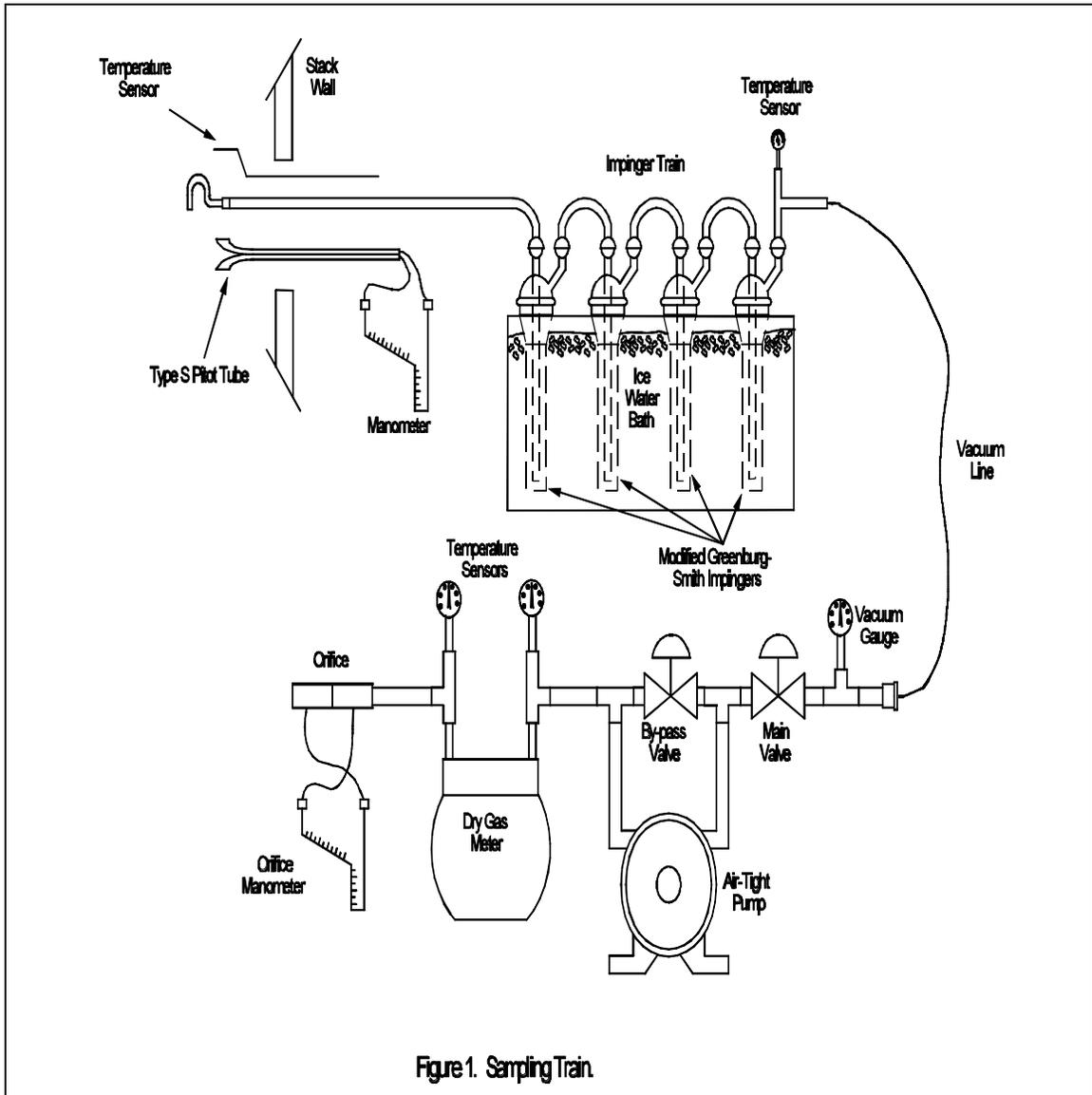
The sampling train consists of the following components: probe nozzle, probe liner, pitot tube, differential pressure gauge, impingers, metering system, barometer, and gas density determination equipment.
